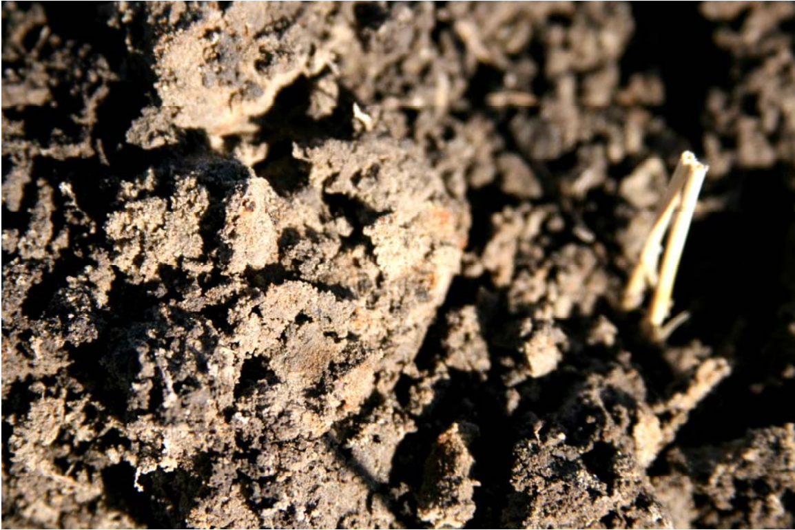
Photo 5: This image shows a close up view of the soil from the B1 horizon from Soil Pit SP-1, which was developed within the wetland area (see Figure 3 for location). The orange mottling is clearly visible in the soil indicating the presence of soil moisture within the upper 12" of the soil column and resulting in the classification of the soil as a hydric soil.
