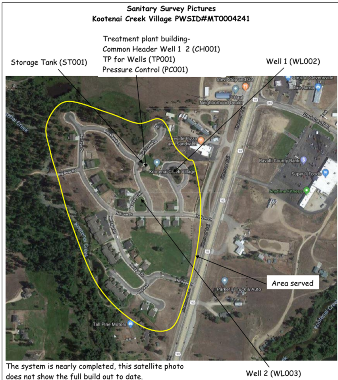
FIGURE 7. KCV WATER SYSTEM (APPENDIX A)
