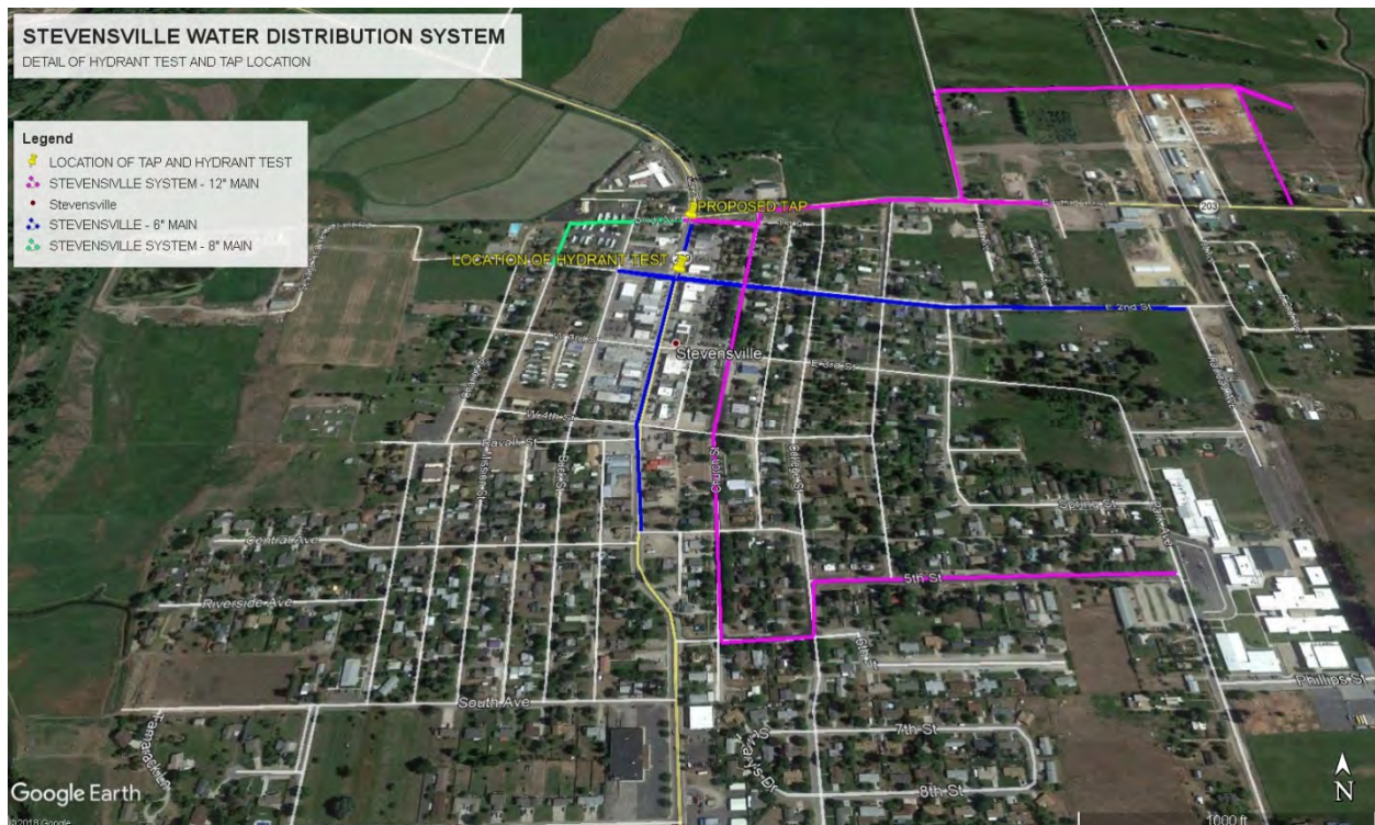
FIGURE 8. STEVENSVILLE EXISTING WATER SYSTEM AND PROPOSED TAP
