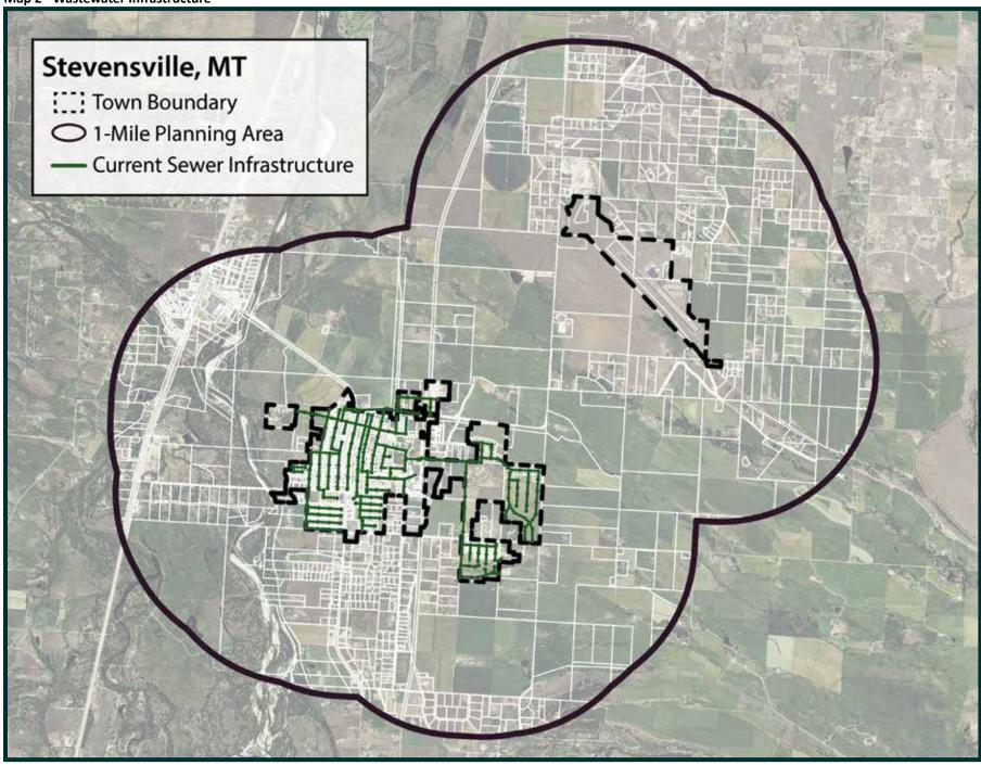
treatment system is estimated to be able to serve 1,007 connections or a population of 2,326. Based on these figures Stevensville's wastewater treatment system could accommodate an additional 224 connections or a population of 517.
